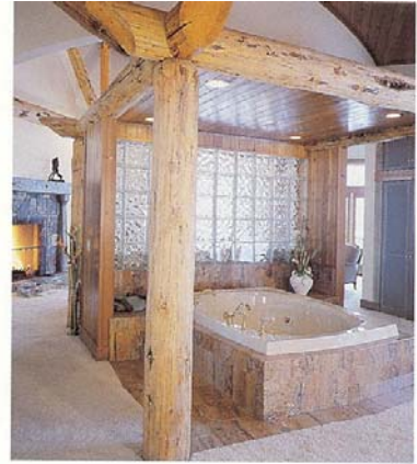
Below: See-through fireplace with birch log mantles serves dining room and sitting room, opposite side. Glue-laminated log beams on ceiling are original square beams reinforced on each side with steel and disguised in a round shape with cedar bark.
